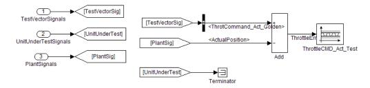
A test harness compares control algorithm simulation results against *golden data* — test results that exhibit the desired behavior for the control algorithm as certified by an expert. In the Verification subsystem, an Assertion block compares the simulated throttle value position from the plant against the golden value from the test harness. If the difference between the two signals is greater than 5%, the test fails and the Assertion block stops the simulation.
