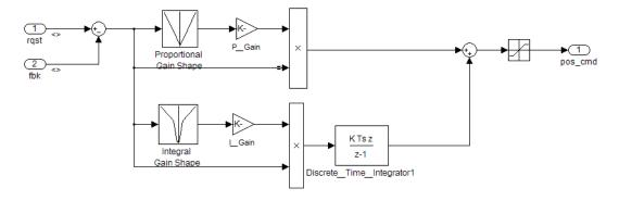
The PI controllers in the model are from a *library*, a group of related blocks or models for reuse. Libraries provide one of two methods for including and reusing models. The second method, model referencing, is described in "Understanding the Simulation Testing Environment" on page 2-8. You cannot edit a block that you add to a model from a library. You must edit the block in the library so that instances of the block in different models remain consistent.
