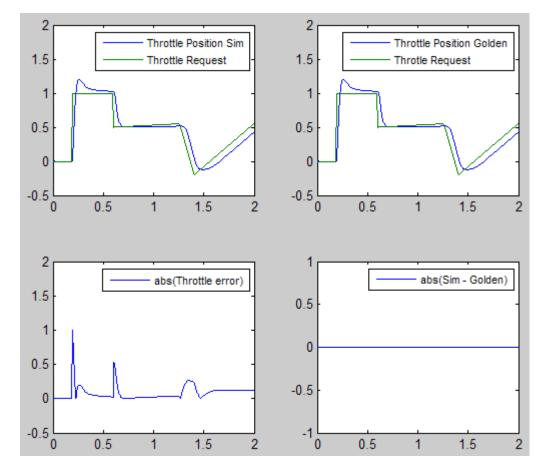
The resulting plot shows that the difference between the golden and simulated versions of the model remains zero.
