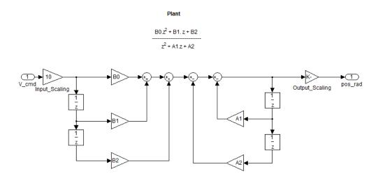
The Plant subsystem models the throttle dynamics with a transfer function in canonical form. You can create plant models to any level of fidelity. It is common to use different plant models at different stages of testing.
