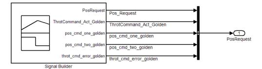
The subsystem uses a Signal Builder block for the test vector source. The block has data that drives the simulation (PosRequest) and provides the expected results used by the Verification subsystem. This example test harness uses only one set of test data. Typically, you create a test suite that fully exercises the system.
